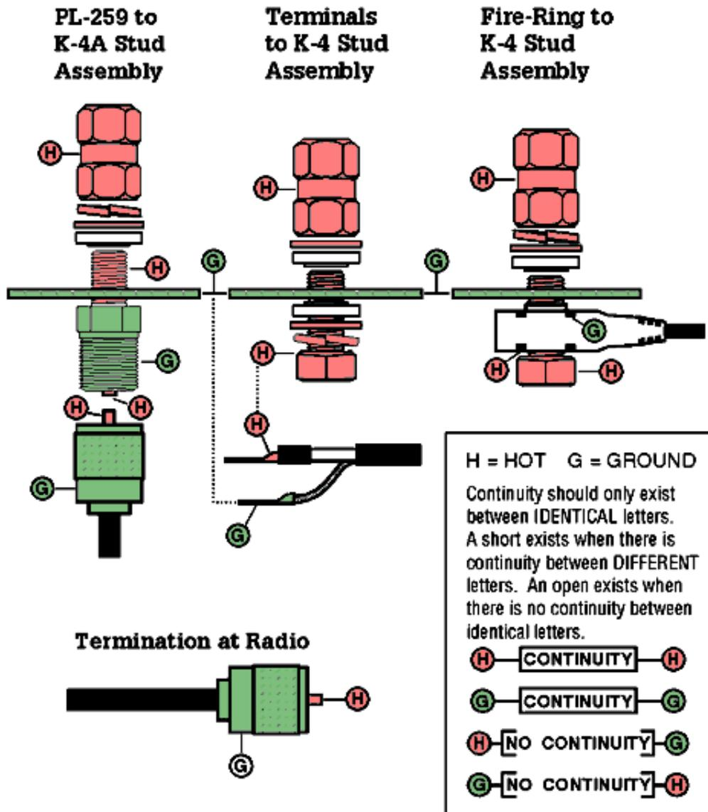
\* System includes CB radio, coaxial cable, primary mount, stud mount, spring or quick disconnect, antenna, and vehicle or ground plane source.
