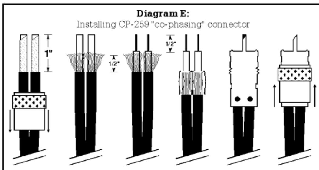
NOTE: If you will be using grommets to protect your cable where it passes through the vehicle body, make sure the grommets are on the cable before processing connector(s).
